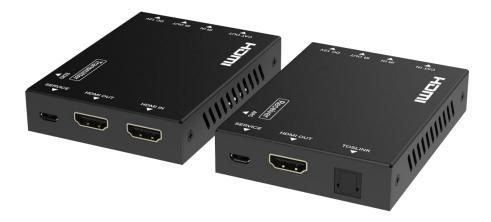
This 18Gbps HDMI Video Extender can extend HDMI signals and IR control signal up to 70m (230 feet) via a single CAT6/6a cable, achieving zero-delay, uncompressed long-distance transmission between the Transmitter and Receiver. The video resolution supports up to 4K@60Hz. It features EDID copy pass-through functionality between the source device and display device, as well as PoC functionality. This Extender is ideal for use in multimedia conference halls, TV teaching, and large-screen displays.
