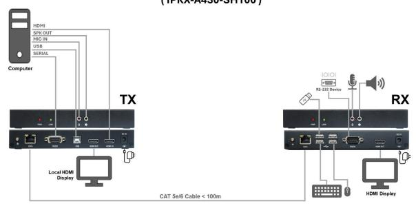
**Note:** The 100m distance can be extended using a 1GbE Unmanaged Switch or Hub. However, only 1 pair of TX-RX extenders can be on the network.
