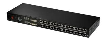
The **RKS-FHDI-CX232** model is ideal for mid-size setup and SME. This model allows dual-user operation over up to 32 servers/computers.
