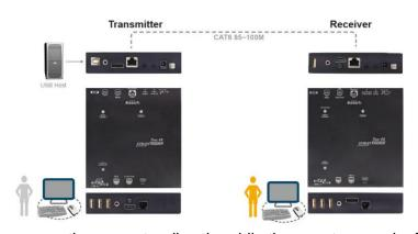
Dedicated USB-A ports on the TX and RX of the Extender units are suitable for both local and remote USB peripheral access. The dual console function allows two users (local and remote) to share one computer. The local console. Transmitter, enables users
