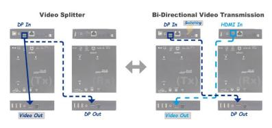
Bi-directional DP/HDMI signal transmission, combined with video switch or splitter functions, enables the video output port on the Transmitter unit (Local Out) to present either local video from the TX or remote video from the RX.
