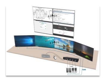
The Mouse Roaming Switching Function allows users to switch among computers by moving the mouse cursor across screen borders, providing a more effective and modern method of computer switching. Users can switch PC ports smoothly and seamlessly by moving the mouse cursor across monitor borders, enabling them to switch keyboards, mice, audio, and USB devices to another PC without using hotkeys or buttons.
