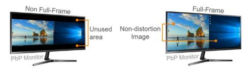
The Switch unique Full-Frame PBP function allows video sources to be displayed on a PBP (Picture by Picture) monitor in full-screen mode, utilizing the entire monitor space. This feature enables two desktop screens to be evenly and entirely displayed on the PBP monitor without distortion or black borders, ensuring a seamless viewing experience.
