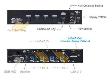
The 4-port KVM Multiview Switch supports not only USB HID keyboard and mouse operation but also USB 3.2 peripheral sharing without any software or driver installation. A unique tracking system enables independent operation of audio and USB devices, which is useful for listening to music or transferring file data from one PC while operating another.
