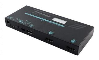
The EDID Mixing Function of VSP-4KH-1H2H is particularly useful in supporting multiple video outputs. This function collects EDID data from all connected displays, mixes them, and creates an optimized EDID that ensures better compatibility and performance across all displays. As a result, all connected displays will function properly and display video accurately.
